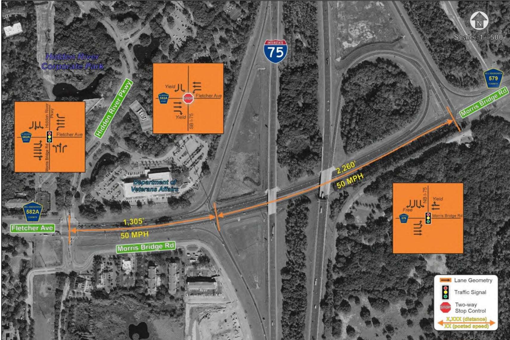
Figure 3: Existing Roadway Characteristics
