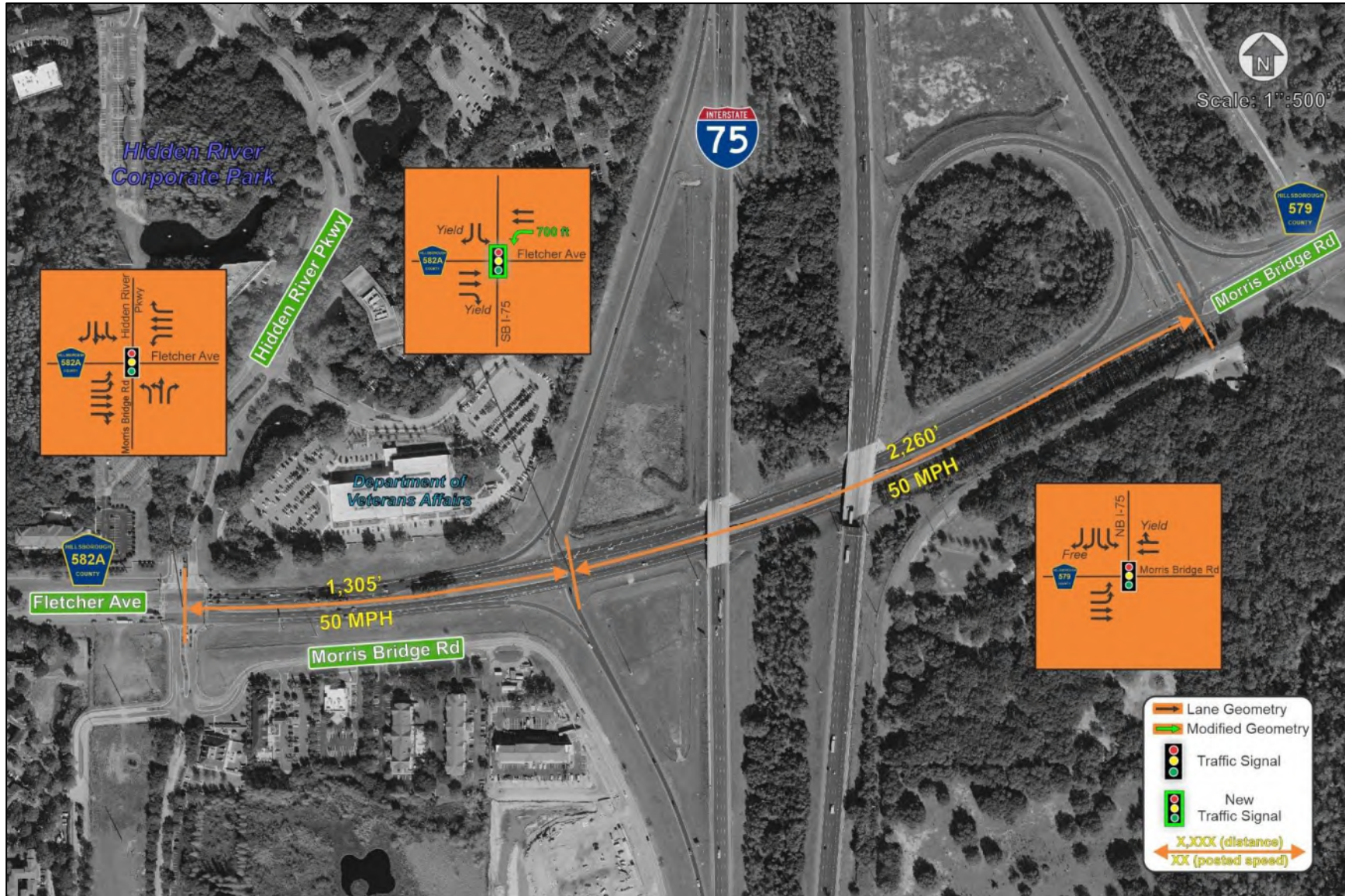
Figure 16: Build Alternative Lane Geometry and Traffic Control
